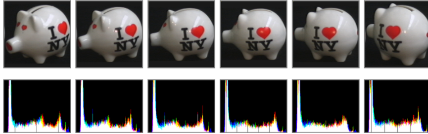
Figure 3.7 Color histograms as perspective invariant features: the same object results in different images when viewed from different viewpoints. Nearly the same parts occur, but in different locations. The images differ when treated as vectors, but their color histograms are almost identical. Images: Colorado Object Image Library [Nene et al., 1996]
